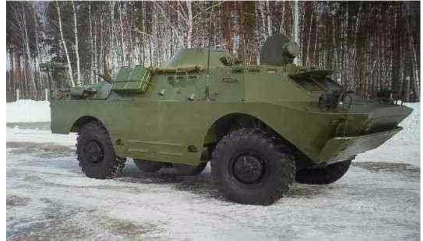
БРДМ - 2 рхб Armoured reconnaissance and patrol vehicle, BRDM - 2 rhb
