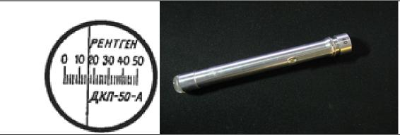
The dosimeter is carried in the pocket of your clothes during operation. Periodically observing through the eyepiece of the dosimeter, determine the value of the dose of gamma radiation received during operation by the position of the thread image on the scale. At the end of the work, the dosimeter is returned to take a reading. To determine the received radiation dose from the readings of the dosimeter, subtract the value of its self-discharge during operation.
